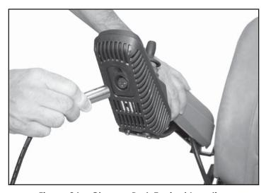
Figure 2A - Charger Port, Typical Location
