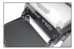
Figure 6A - Footrest Adjustment Screws
