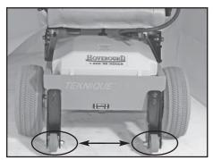
Figure 5A RWD and GT Anti-Tip Wheels (Rear Wheel Drive Shown)
