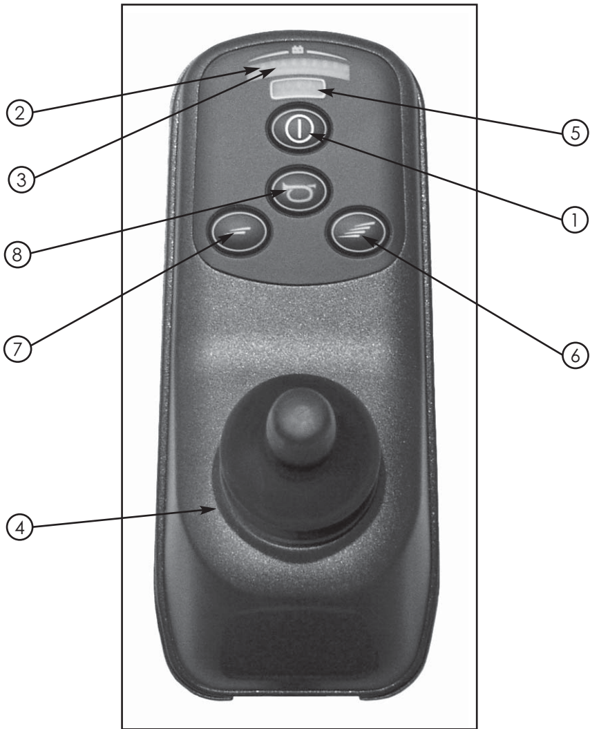
Figure 1A- VSI Controller
