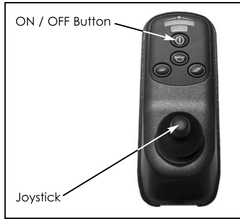
Figure 9A - VSI Controller and new VSI Controller
